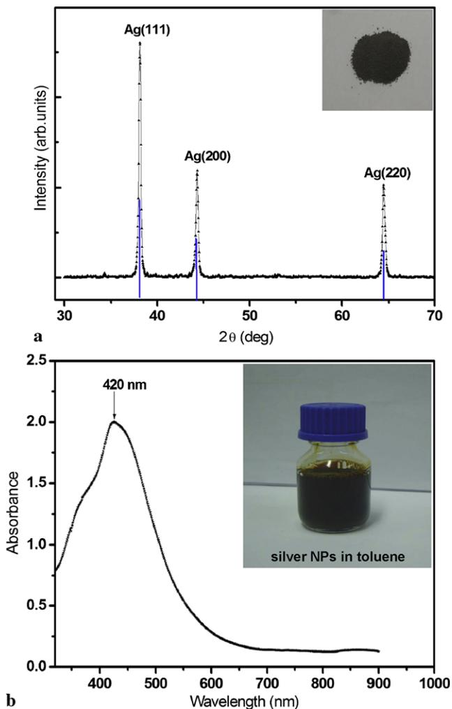
**Fig. 3** (a) X-ray diffraction pattern of the silver NPs. Inset is a photograph showing a paper containing as-synthesized silver NPs. (b) UV-vis spectrum of silver NPs in toluene
