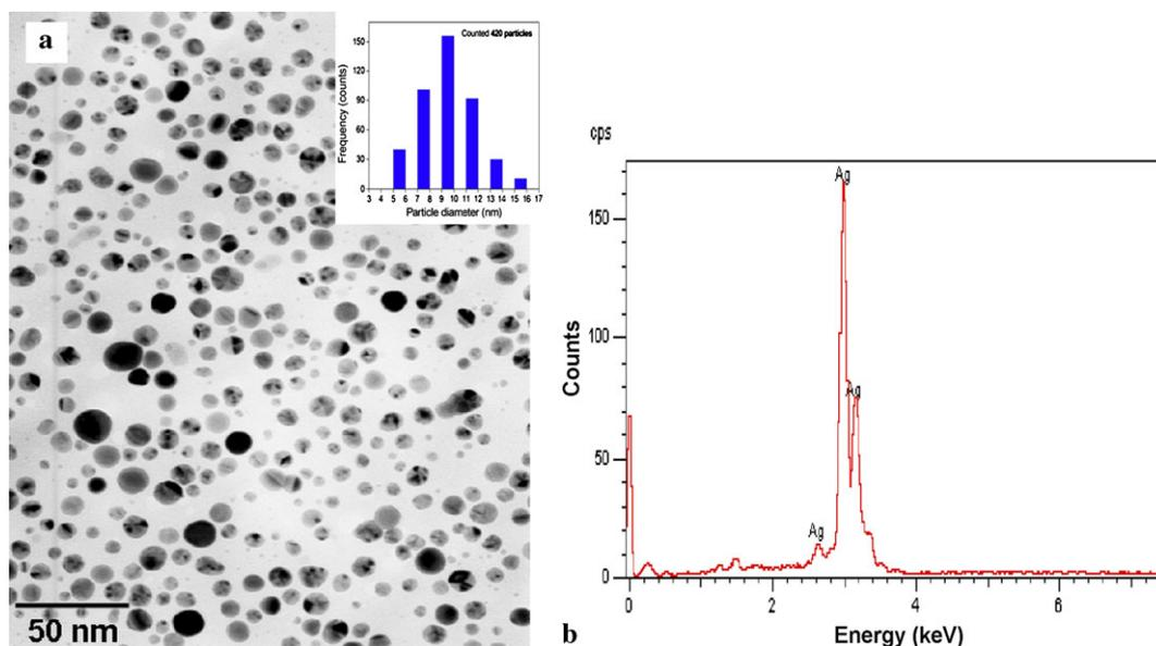
**Fig. 2** (a) Transmission electron microscopy image and size distribution of the as-prepared silver NPs; (b) An energy-dispersive X-ray spectrum of prepared silver NPs
