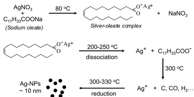
**Fig. 1** Illustration for synthesis of silver NPs by using a thermal decomposition method. The silver-oleate precursors were prepared from the reaction of the silver nitrate and sodium oleate. The thermal decomposition of the silver-oleate complex produced the silver NPs with average particle size about 10 nm
